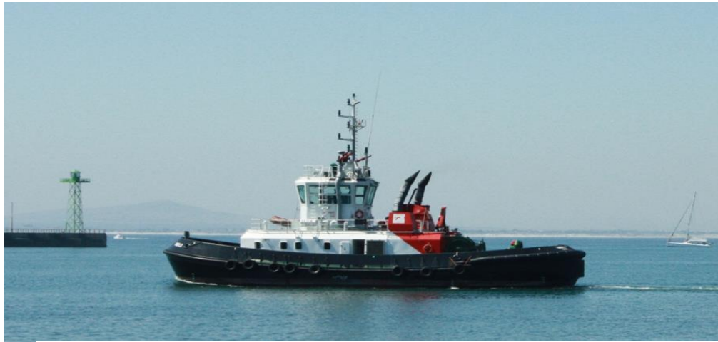
The omni-directional harbour tug Umbilo, one of nine similar tugs built in Durban in a tug replacement programme (the fourth such building programme involving omni-directional tugs) for South African ports and concluded in 2020.
